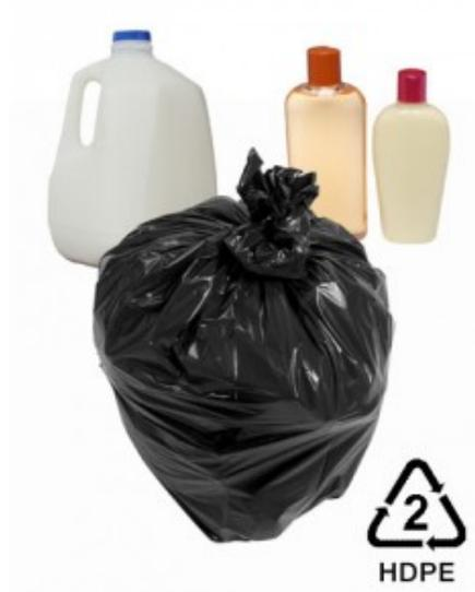
HDPE is a versatile plastic with many uses, especially for packaging. It carries low risk of leaching and is readily recyclable into many goods.
